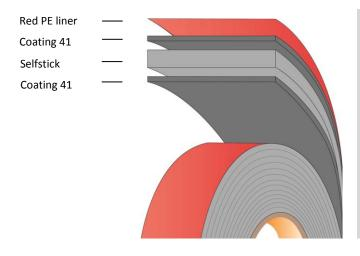
Thickness: 1.2mm  $(0.047 \text{ inch}) \pm 10\%$ Core: Conformable acrylic
